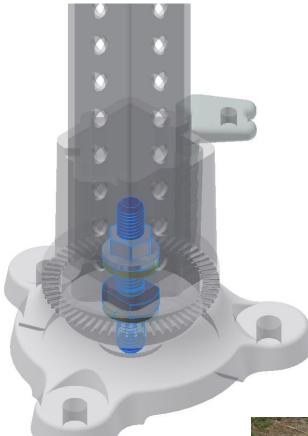
• Product is a 360 degree index-able, surface mountable sign post coupler for Perforated Square Steel Tube sign posts.
